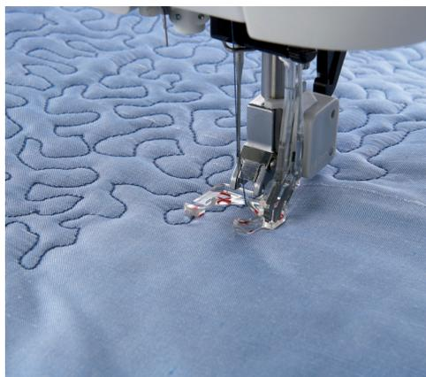
Touch Sensormatic free-motion setting to set the machine for Sensormatic free-motion mode with presser foot 6A.
