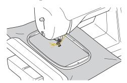
Remove the thread for the first color from the machine. Thread the machine with the next color.
