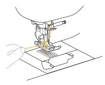
Pull up the bobbin thread, pass it under the presser foot and pull it about 10 cm (4 inches) toward the back of the machine, making it even with the upper thread.
