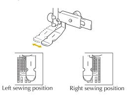
Change the needle position so that the needle does not touch the presser foot.
