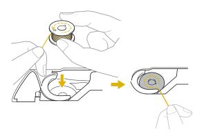
Lightly hold down the bobbin with your right hand (1), and then guide the end of the thread around the tab of the needle plate cover with your left hand (2).
