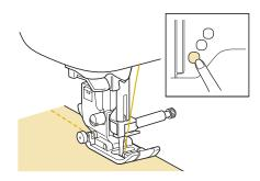
Press  $(\approx)$  (Thread cutter button) to trim the upper and lower threads.
