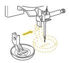
Tighten the screw with the included screwdriver.
