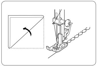
Use a lightweight fabric such as tricot. Fold the fabric and stitch on the bias. You may need to increase the needle thread tension slightly. Allow the needle to just clear the folded edge of the fabric at zigzag stitches.
