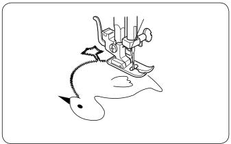
Baste (or fuse with iron-on fabric joiner) appliqué onto the fabric.
