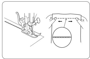
The stitch is sewn with two forward stitches and one reverse stitch, creating a seam that is difficult to tear.
