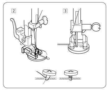
2 Match the holes in the button with the horizontal slot on the presser foot.
