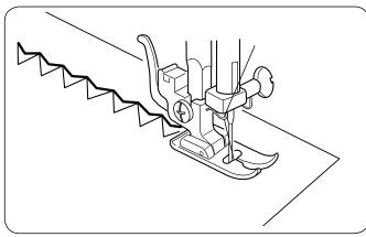
The balance must be adjusted if the nature of the fabric prevents a uniform forward and backward feed. To do so, turn the stitch length knob as follows:
