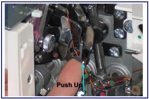
Tugging slightly on the thread tail at the back of the serger, push the threader lever all the way up to hook thread into the eye at the back of the looper.
