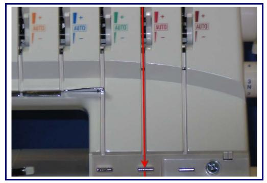
Lay the thread through Red tension disk while holding the thread securely with both hands. Next slip into guide directly below the tension from right to left.
