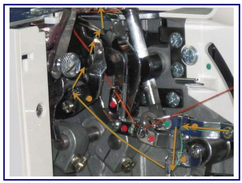
Using the tweezers thread the last thread guide that is located on the left just below the looper. Next thread the brown looper eye from front to back, pulling the thread over the top of the red looper, then pull the thread tail to the back of the serger approximately 4 to 6 inches. Make sure the thread sits over the top of the V cut out just before the eye of the looper. (See page 21 illustration 10 of your manual.)
