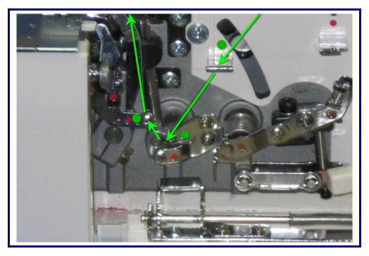
Using tweezers slip the thread into the next three guides marked with the small green dots.
