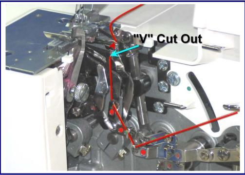
Thread the eye of the looper as shown, making sure that the thread is positioned in the "V" cutout in front of the looper. Pull the thread tail to the back of the serger approximately 4 to 6 inches.
