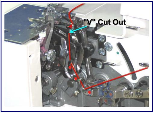
Thread the eye of the looper as shown, making sure that the thread is positioned in the "V" cut out in front of the looper. Pull the thread tail to the back of the serger approximately 4 to 6 inches.
