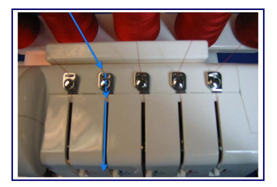
Thread the top cover guide by slipping the thread under the guide from right to left, and then pull the thread under the small round disk from the right side.
