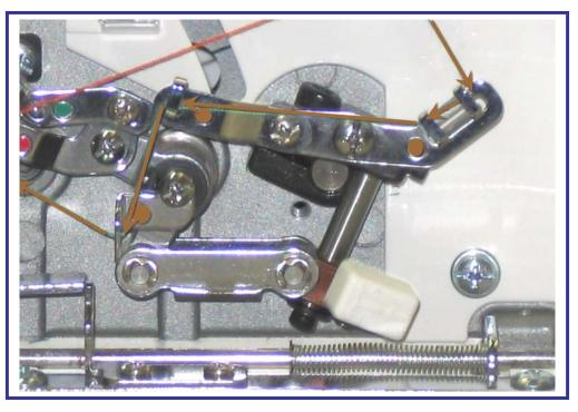
Using the tweezers thread the next 4 guides identified with a small brown dot.
