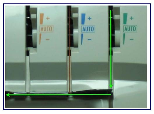
Lay thread through Green tension disk, while holding the thread securely with both hands. Next slip into guide directly below the tension from right to left.
