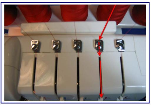
Thread the top thread guide by slipping the thread under the guide from right to left, and then pull the thread under the small round disk from the right side.
