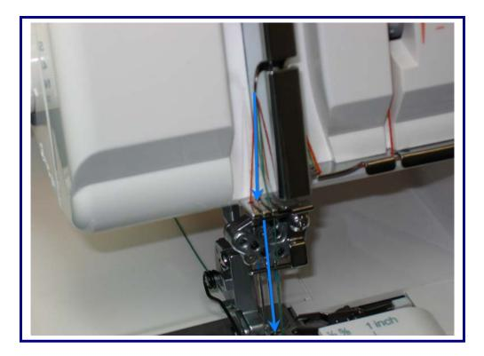
Slip the thread into the center slot.
