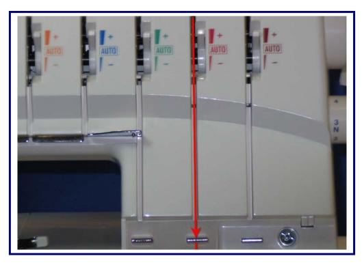
Lay thread through Red tension disk while holding the thread securely with both hands. Next slip into guide directly below the tension from right to left.
