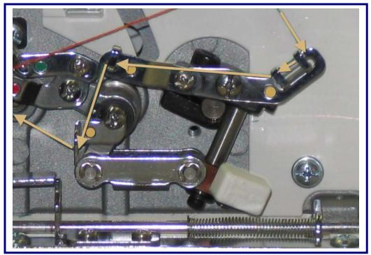
Using tweezers thread the next 4 guides identified with a small brown dot.
