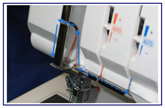
Slip the thread into the third slot closest to the back and then up and over the take up lever slot.
