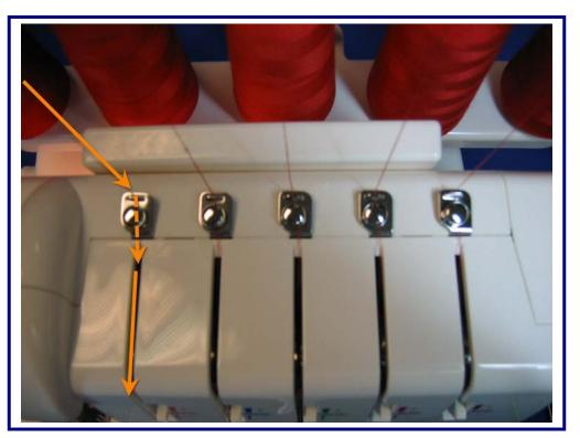
Thread the top cover thread guide by slipping the thread under the guide from right to left, and then pull the thread under the small round disk from the right side.
