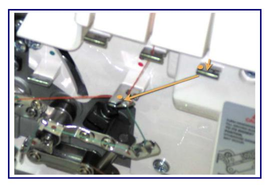
Slip thread through front slot of threading guide.
