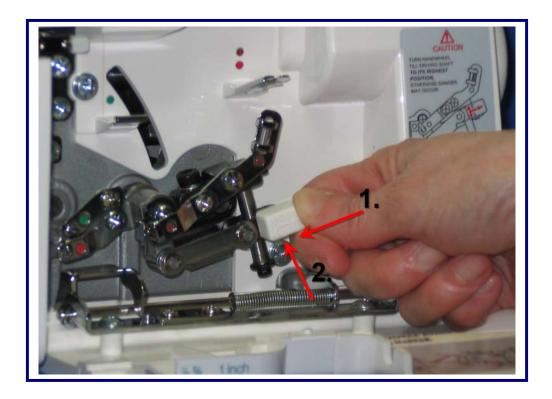
To lower looper push the knob all the way to the left and then push upwards.
