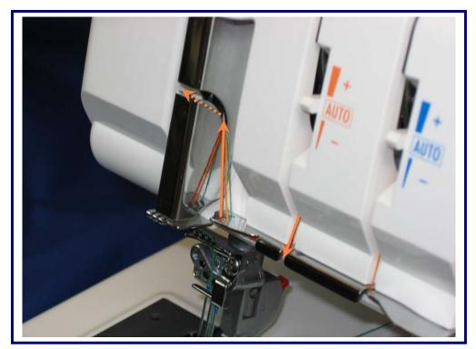
Slip thread into the first slot and then into the take-up lever slot.
