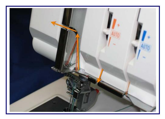
Slip the thread into the center slot and then up and over the take-up lever slot.
