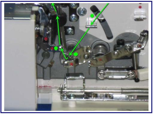
Using tweezers slip the thread into the next three guides marked with small green dots.
