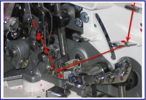
Using tweezers slip the thread into the slot at the back of the thread guide, and then into the next three guides marked with the small red dots.
