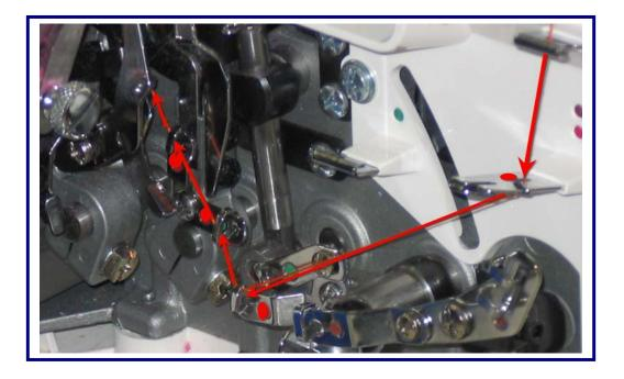
Using tweezers slip the thread into the slot at the back of the thread guide, and then into the next three guides marked with the small red dots.
