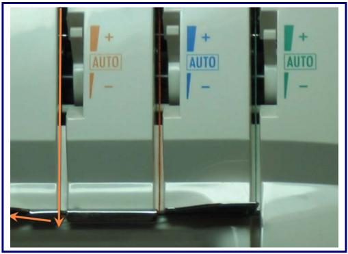
Lay thread through Orange tension disk, while holding the thread securely with both hands. Next slip into guide directly below the tension from right to left.
