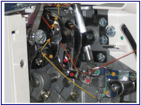
Using the tweezers thread the last thread guide that is located on the left just below the looper. Next thread the brown looper eye from front to back, pulling thread over the top of the red looper, then pull the thread tail to the back of the serger 4 to 6 inches. Make sure the thread sits over the top of the "V" cut out just before the eye of the looper. (See page 21 figure 10 of your manual.)
