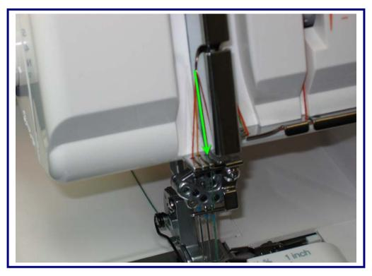
Slip the thread into the third slot closest to the take-up lever.
