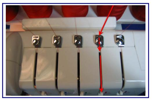
Thread the top cover thread guide by slipping the thread under the guide from the right to left, and then pull the thread under the small round disk from the right side.
