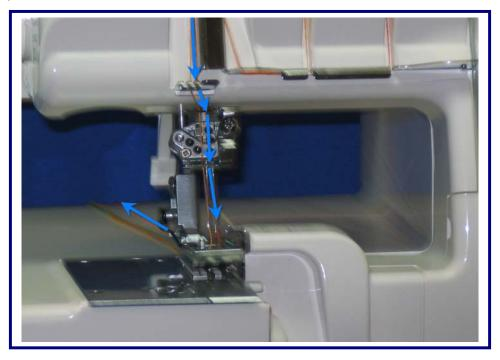
Slip the thread into the third slot on the right next to the take-up lever, then into the third slot on the right in the guides just above the needle clamp. Next slip the thread behind the metal guide and then into the eye of the needle in (B) position, and then under what looks like a bridge at the back of the foot. Pull the thread tail to the back of the serger.
