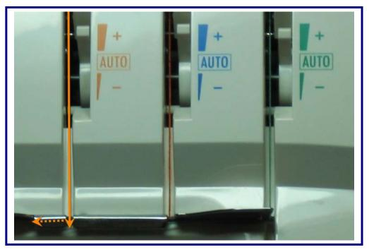
Lay thread through Orange tension disk, while holding the thread securely with both hands. Next slip into guide directly below the tension from right to left.
