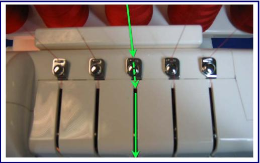
Thread the top cover thread guide by slipping the thread under the guide from right to left, and then pull the thread under the small round disk from the right side.
