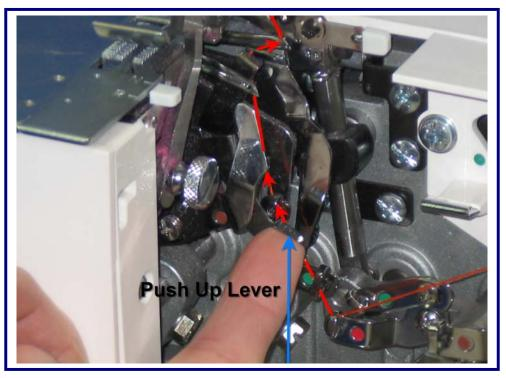
Tugging slightly on the thread tail at the back of the serger, push threader lever all the way up to hook thread into the eye at the back of the looper.
