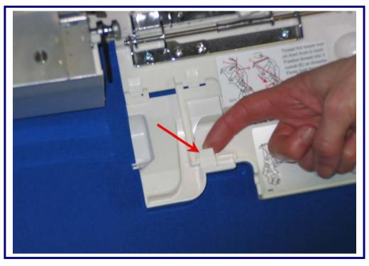
Remove the knife cover (overedge plate) by gently raising the lever as shown and pulling the cover towards you.
