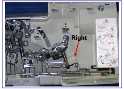
In order to attach the Cover Plate, you must first disengage the upper looper.
