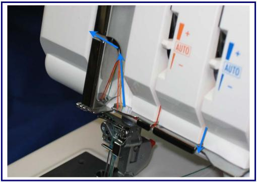
Slip the thread into the third slot closest to the back and then up and over the take-up lever slot.
