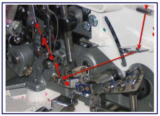
Using tweezers slip the thread into the slot at the back of the thread guide, and then into the next 3 guides marked with small red dots.
