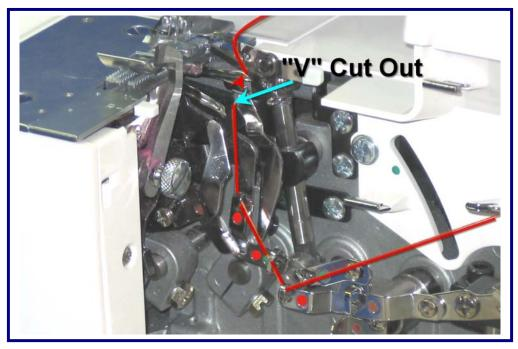
Thread the eye of the lower looper as shown, making sure that the thread is positioned in the V cut out in front of the looper threader. Pull the thread tail to the back of the serger approximately 4 to 6 inches.
