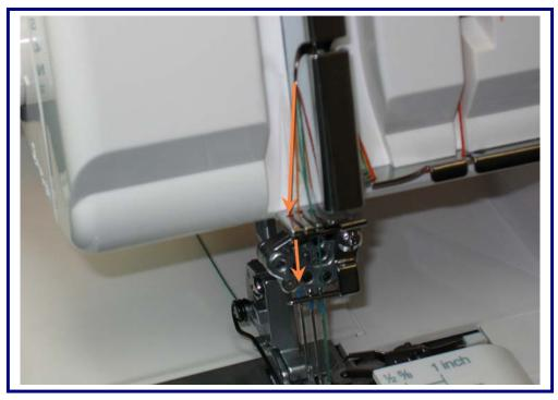
Slip the thread into the first slot.
