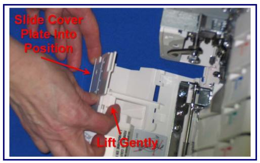
Slip the Cover Stitch Plate onto the front cover by raising the lever as shown and pushing the plate towards the machine until it snaps into place.
