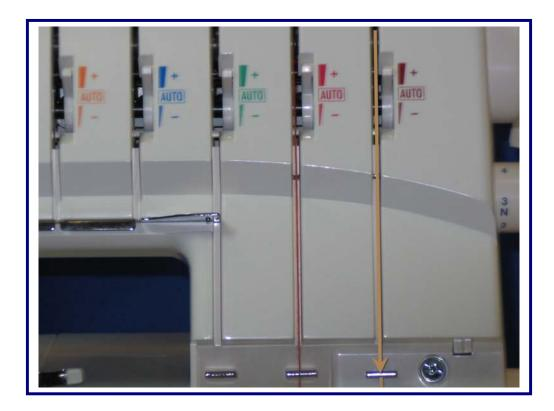
Lay thread through Brown tension disk, while holding the thread securely with both hands. Next slip into guide directly below the tension from right to left.
