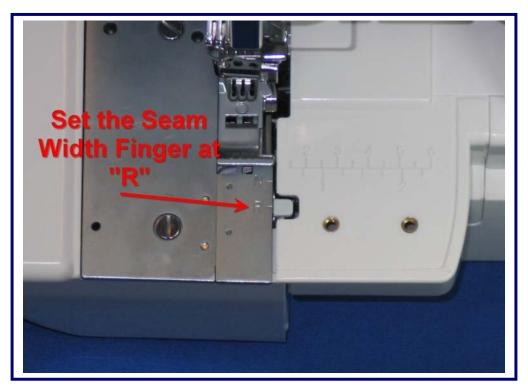
In order for the Cover Stitch Plate to sit properly, you must set the seam width finger to the "R'' position.
