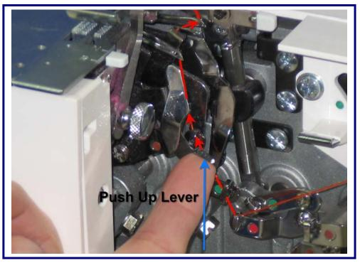
Tugging slightly on the thread tail at the back of the serger, push threader lever all the way up and to the left to hook the thread into the eye at the back of the looper.
