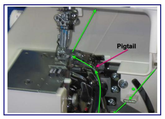
Thread the guide that looks like a little pigtail and then thread through the eye of the looper as shown. Pull the thread tail to the back of the serger approximately 4 to 6 inches.
