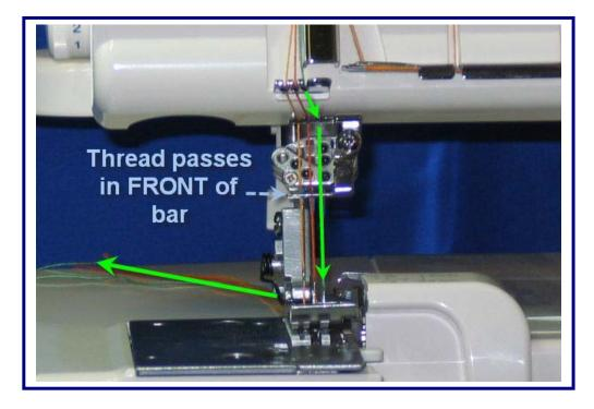
Slip thread through third slot on the right; next slip it in front of the thread guide and then into the eye of the needle (E) on the right. Finally thread the tail of the thread through the opening in the foot directly below the needle; pull thread under the foot and to the back of the serger.
