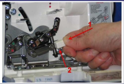
To lower the looper push the knob all the way to the left and then push it up. (*To re-engage the looper push the knob all the way to the left and push it down. Turn the handwheel towards you to raise the looper.*)
