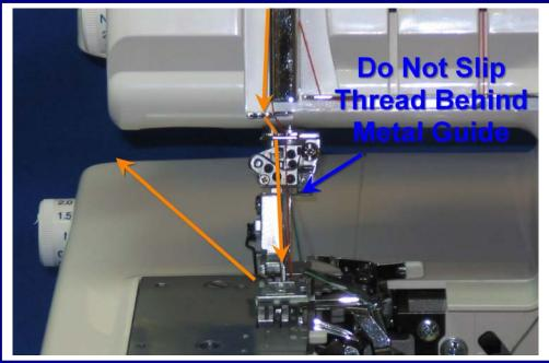
Slip the thread into the center slot next to the take-up lever, then into the center slot in the guides just above the needle clamp. Next slip the thread in front of the metal guide and then into the eye of the needle in (D) position, through the opening in the foot and then pull the thread tail to the back of the serger.
