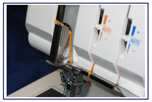
Slip the thread into the center slot and then up and over the take-up lever slot.
