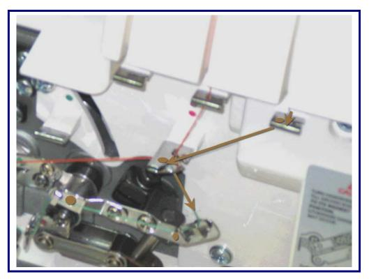
Slip thread through front slot of thread guide.
