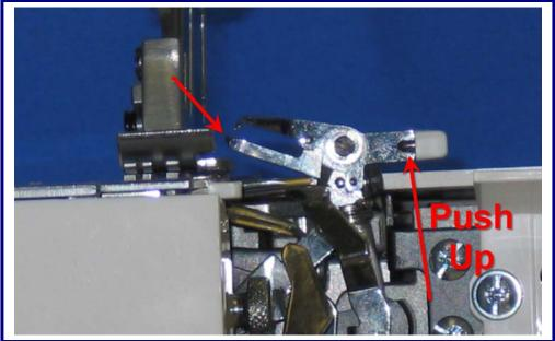
Push white spreader lever up so that spreader slips into the eye of the looper.
