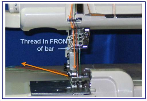
Slip thread through first slot on the left; next slip it in front of the thread guide and then into the eye of the (C) needle on the left. Finally thread the tail of the thread through the opening in the foot directly below the needle, pull thread under the foot and to the back of the serger.
