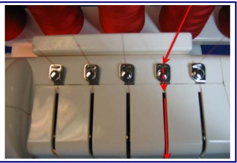
Thread the top cover thread guide by slipping the thread under the guide from right to left, and then pull the thread under the small round disk from the right side.
