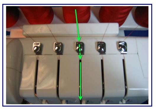
Thread the top cover thread by slipping the thread under the guide from right to left, and then pull the thread under the small round disk from the right side.
