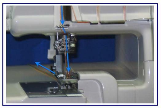
Slip the thread into the third slot on the right next to the take-up lever, then into the third slot on the right in the guides just above the needle clamp. Next slip the thread behind the metal guide and then into the eye of the needle in B position, and then under what looks like a bridge at the back of the foot. Pull the thread tail to the back of the serger.
