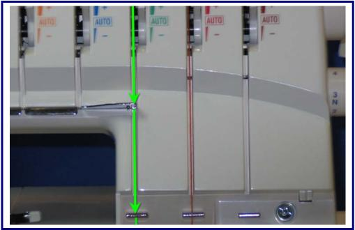
Lay thread through Green tension disk, while holding the thread securely with both hands. Next slip into guide directly below the tension from right to left.
