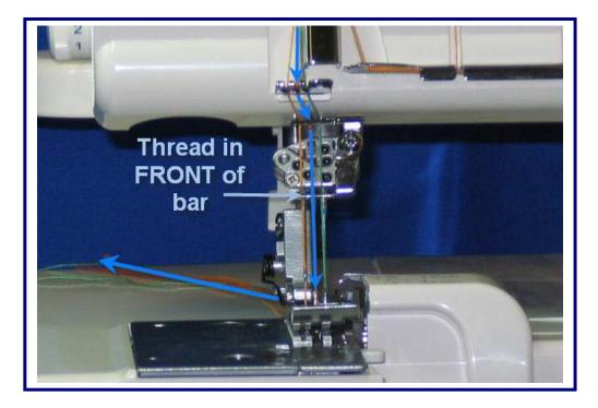
Slip thread through center slot; next slip it in front of the thread guide and then into the eye of the center (D) needle. Finally thread the tail of the thread through the opening in the foot directly below the needle, pull thread under the foot and to the back of the serger.
