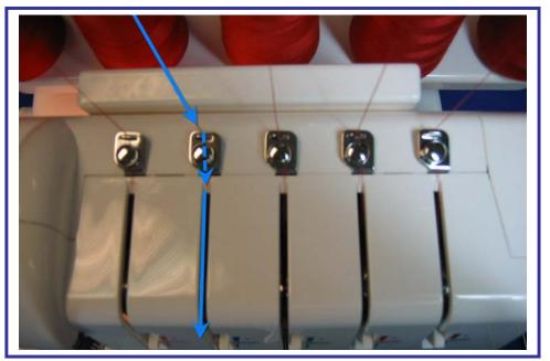
Thread the top cover thread guide by slipping the thread under the guide from right to left, and then pull the thread under the small round disk from the right side.
