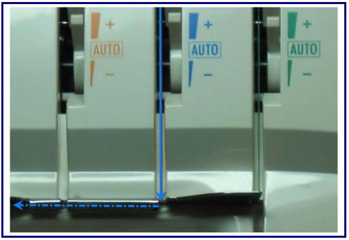
Lay thread through Blue tension disk while holding the thread securely with both hands. Next slip into guide directly below the tension from right to left.
