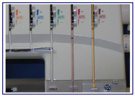
Lay thread through Brown tension disk while holding the thread securely with both hands. Next slip into guide directly below the tension from right to left.
