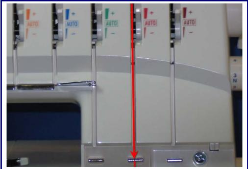
Lay thread through Red tension disk while holding the thread securely with both hands. Next slip into guide directly below the tension from right to left.
