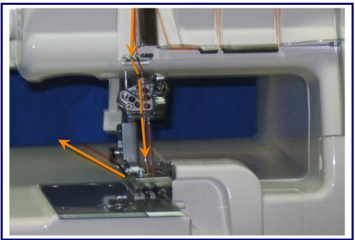
Slip the thread into the center slot next to the take-up lever, then into the center slot in the guides just above the needle clamp. Next slip the thread behind the metal guide and then into the eye of the needle in A position, and then under what looks like a bridge at the back of the foot. Pull the thread tail to the back of the serger.
