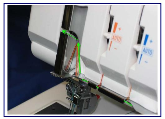
Slip the thread into the third slot at the back and then into the take-up lever slot.
