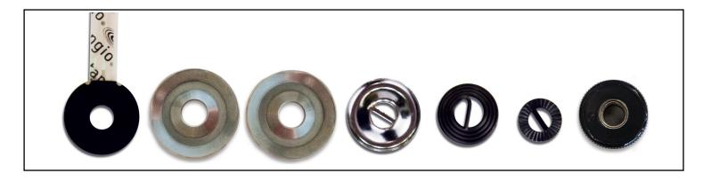
**STEP 4:** Remove all components from the tension guide, including both tension discs. Place each part in the order you removed them. This makes it much easier to put everything back together.
