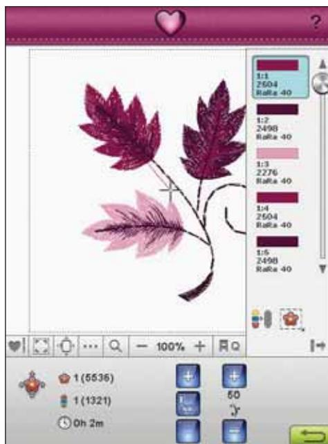
6. Clear sufficient space around the machine to accommodate movement of the embroidery arm and the hoop. Hold the needle thread and press the Start/Stop button or the foot control. The machine starts embroidering.
