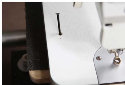
Figure 38 Oil dip stick lifted
