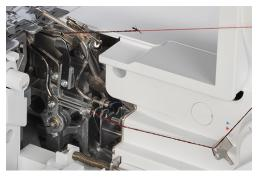
> Place the looper threads under the presser foot to the rear left.
