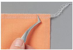
> Pull the needle thread out of the seam.
