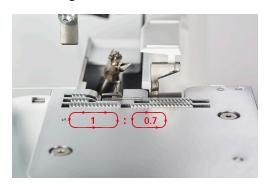
The front feed dog (0.7) covers a shorter distance than the rear feed dog (1). The material is stretched under the presser foot which helps to reduce puckering. This setting can also be used to deliberately stretch the material.
