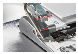
> Lower the presser foot shaft carefully until the shaft groove engages with the presser foot pin.
