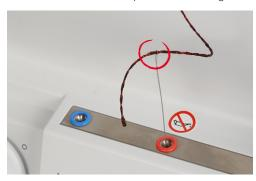
> Pull the end of the threading wire until the looper thread emerges from the eye of the looper.
