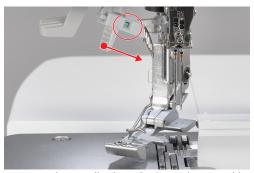
> Press the needle threader lever down and keep pressed.
