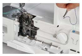
> Pull the auxiliary thread ends until the thread comes out of the looper eye.
