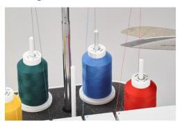
> Tie the inserted looper thread to the new thread.
