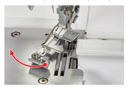
> To set the presser foot in the sewing position, lower the presser foot lifter or swing the presser foot sideways to the right.
