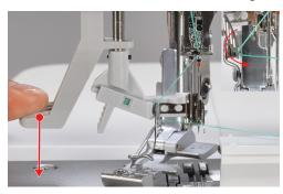
> Release the pressure on the needle threader selector and let it go back to its initial position.
