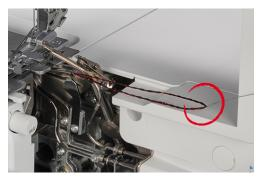
> Place the looper threads under the presser foot to the rear left.
