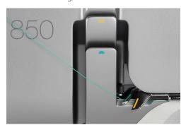
> Place the thread over the upper needle thread take-up lever cover and pull it down.
