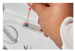
> Pull a thread reserve of approx. 40 cm so that the thread can be completely drawn through the threading path.
