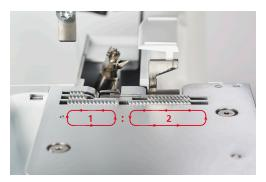
At a setting of 1.5 - 2 the front feed-dog (2) covers a longer distance than the rear feed-dog (1).
