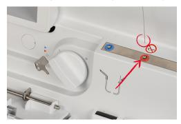
> Place the wanted looper thread through the loop of the threading wire.
