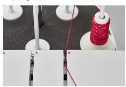
> Place the thread along the slot into the thread tension discs.
