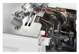
> To minimize the loops of the looper at the fabric edge, turn the mtc micro thread control in «-» direction during sewing.
