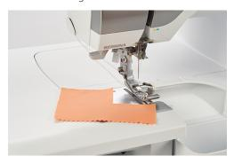
> Sew the seam until the knife reaches the corner.
