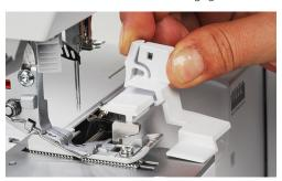
> To remove the seam guide, press the upper part of the clamp together and pull it away from the knife cover insert.
