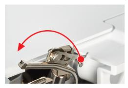
> Lightly press back on the retaining bracket and hook the snap-in lug into the eye of the looper.
