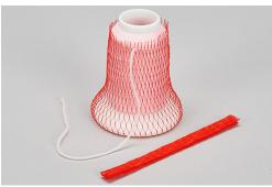
> Slip the spool net from above over the thread spool and pull the thread end up.
