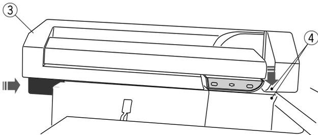
Place the embroidery unit on the back side of the machine base, matching the small dots as shown.
