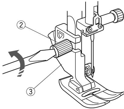
Attach the embroidery foot P to the presser bar from behind. Tighten the setscrew securely.
