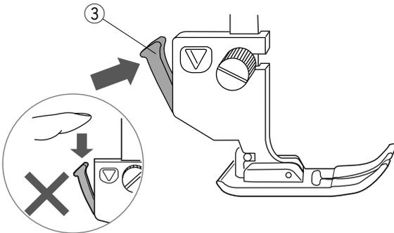
Press the black lever on the backside of the foot holder.
