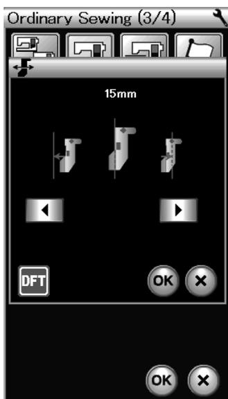
Press the ◀ key or ▶ key to adjust the position of the cloth guide.
