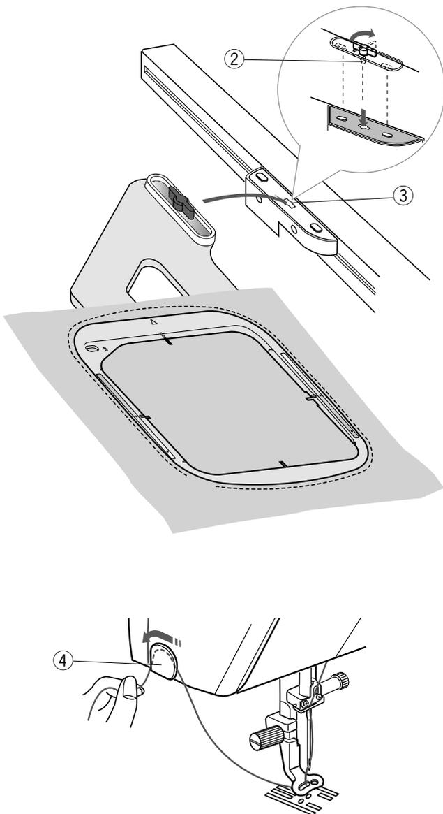
Place the hoop on the machine and attach the hoop to the carriage by inserting the lock pin of the hoop into the hole in the carriage.
