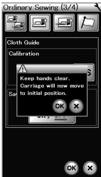
Press the YES key and a warning message will appear. Press the OK key and the carriage will move to the standard position.
