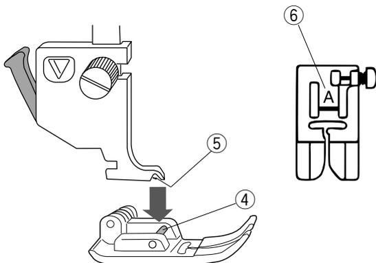
Place the desired foot under the foot holder so that the pin of the foot lies just under the groove of the foot holder.
