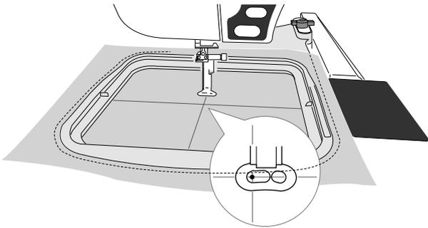
Adjust the hoop position with the jog keys so that the needle position comes right above the center of the centerlines on the fabric.
