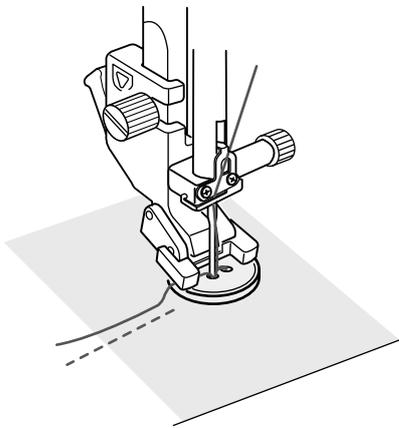
Place a button on the fabric and lower the needle into the left hole of the button by turning the handwheel with your hand.
