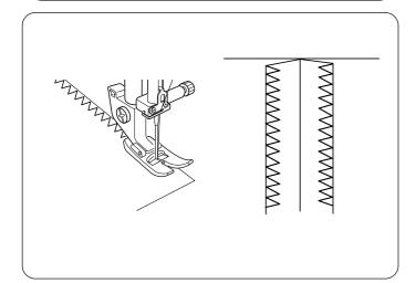
This stitch is useful in garment construction, and in finishing raw edges of any sewing project.
