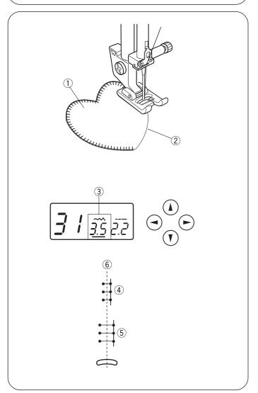
\* The stitch width of pattern 31 – 33 can be changed without changing its center needle position.
