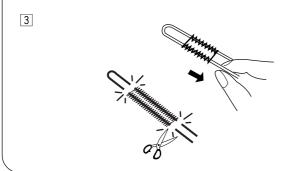
3 Pull the loose ends of the filler cord to tighten it. Thread the end of the cord through a hand-sewing needle. Then draw them to the wrong side of the fabric and knot.
