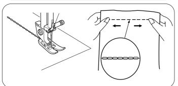
This strong, durable stitch is recommended when both elasticity and strength are necessary in order to insure comfort and durability. Use it to reinforce areas such as crotch and armhole seams. Also use for extra reinforcement when constructing items such as backpacks.
