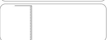
For seaming garments, zipper application and more. Pattern 01 is used for seaming fine fabrics.
