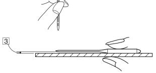
To check needle straightness, place the flat side of the needle onto something flat (a needle plate, glass etc.) The gap between the needle and the flat surface should be consistent.
