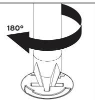
Screw cam bolts flush as illustrated.
