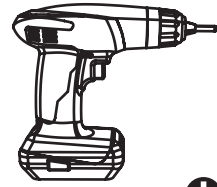
Electric Screwdriver Torque set to 3-5
