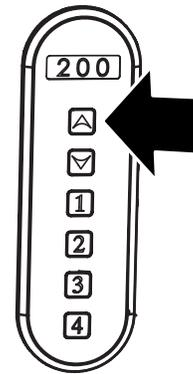
Press and hold the UP button on your controller to position your lift platform in the uppermost position. Press and hold the preset position of your choice for 5 seconds. Free Arm Position is now pre-set.
