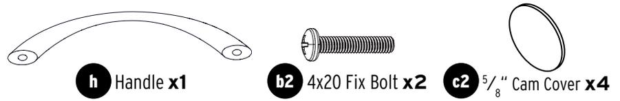
Attach drawer front **Panel L** to drawer side **Panels L3 and L2** as shown, sliding drawer bottom **L7** into the groove on **Panel L**. Then attach **h Handle** with **b2 Fix Bolts**.
