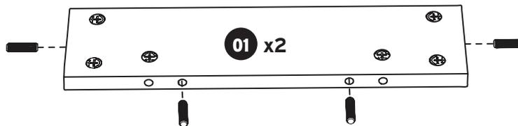
Insert 4 **Dowel Pins** in each of the two **Panel 01** pieces.
