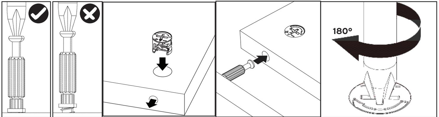
Screw cam bolts flush as illustrated.
