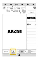
Touch to turn off the thread cutting function and then touch .
