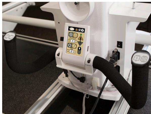
2. The rear handlebars come mounted to a bracket. Line up the two holes in the bracket with those on the rear of the machine.
