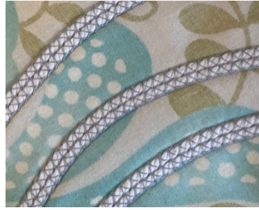
Top and underside view using the Cord Guide Plate and 2.5mm Cording Micro Insert foot with 12wt. cotton thread in each wiper when stitching curves for a decorative look.
