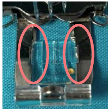
Alignment position for Micro Insert Foot
