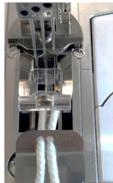
Cording in each guide on the Cord Guide Plate
