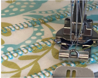
Top and underside view using the Cord Guide Plate and 2.5mm Cording Micro Insert foot with 12wt. cotton thread in each wiper when stitching straight rows for a decorative look.
