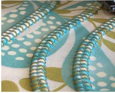
Top and underside view using the Cord Guide Plate and 2.5mm Cording Micro Insert foot with 12wt. cotton thread in each wiper when stitching curves for a decorative look.
