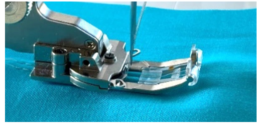
Triple Cover Stitch tested and ready to add the wiper threads.
