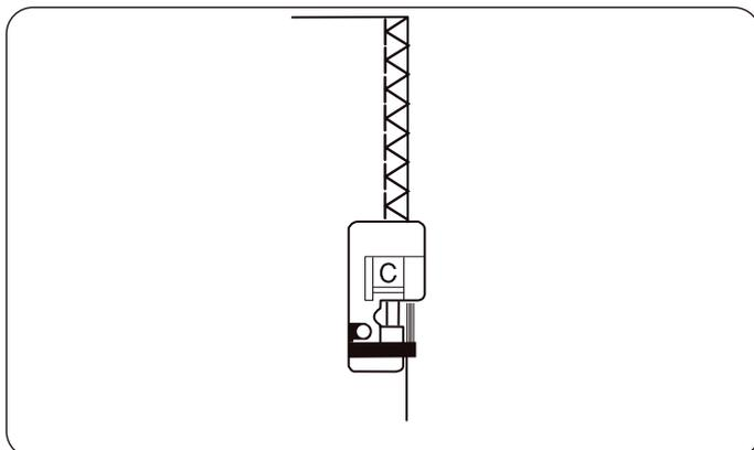
This stitch is used to simultaneously seam and overcast edges of fabrics. Use this stitch when you do not need to open seams flat.
