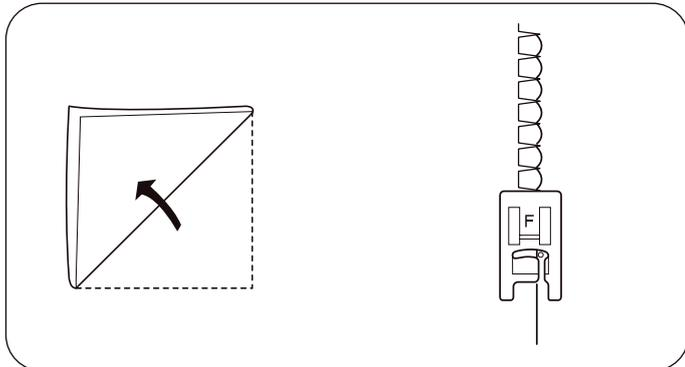
Use a lightweight fabric (tricot, for example). Fold the fabric as shown and stitch on the fold. Allow the needle to just clear the folded edge to create a shelled edge. The thread tension may need to be increased slightly.
