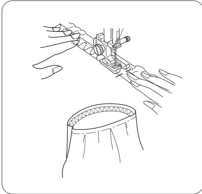
Mark the elastic into quarters. Match those to the center front, center back and side seams, and pin the elastic to the fabric.
