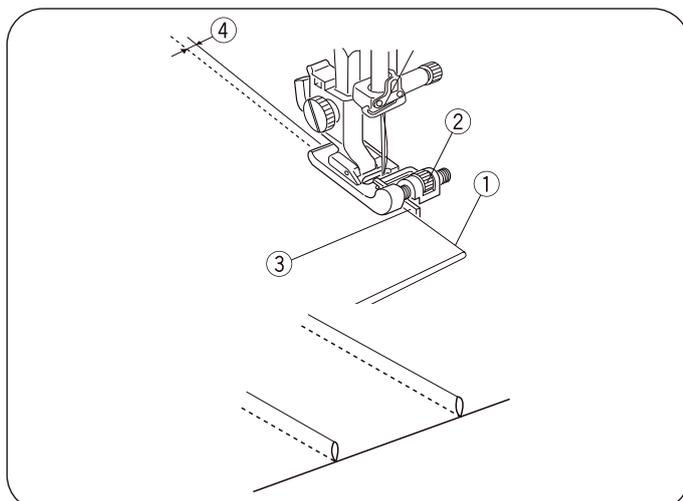
Open the fabric and press the tuck to one side.
