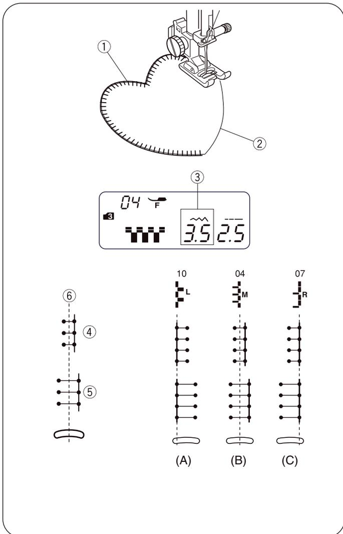
(A) The stitch pattern 10 has a fixed left needle position. When you change the stitch width, the right needle position will change.
