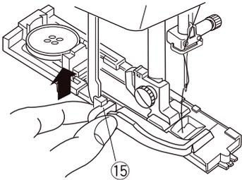
5 Start the machine to sew the buttonhole. The buttonhole will be automatically sewn. The machine will sew the left row first.
