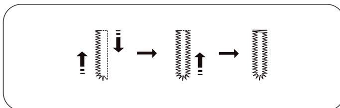
Sewing procedure is the same as standard buttonhole. The stitch width can be varied from 2.5 to 5.5.
