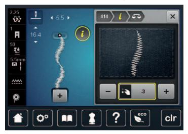
> To correct the longitudinal direction of the stitch pattern, turn the «Lower Multi-function knob» until the preview of the stitch pattern matches the stitch pattern sewn on the fabric.
