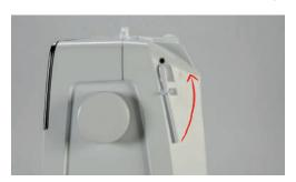
Inserting foam pad and thread spool
