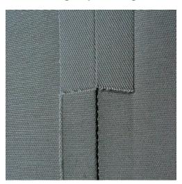
The Triple straight stitch is especially suitable for durable seams and for firm, densely woven fabrics such as denim and corduroy. suitable for durable seams and for firm, densely woven fabrics such as denim and corduroy. For firm or densely woven materials it is recommended to fit the Jeans Foot #8. This will help to sew denim or canvas. For decorative topstitching, the stitch length can be elongated.
