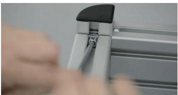
> Insert the spring slot nut from beneath into the groove of the left leg and position it exactly in front of the screw hole.
