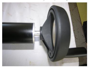
> Insert the handwheel screw through the conical washer into the screw hole and tighten it with the Allen key.
