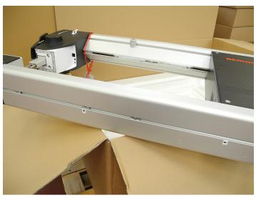
> Unpack the two stand profiles as well as the bag containing the stand profile kit from the packaging of the machine.
