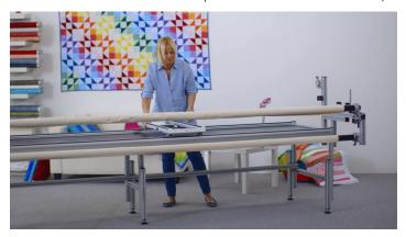
> If necessary, open the screws of the carriage and readjust. If all of the four screws need to be loosened, the carriage has to be aligned parallel to the Frame.
