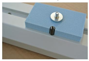
> Now mount the completely prepared front stand profile on the bottom side of the machine. The machine is still lying on its side when doing this. Tighten the screw P11 slightly in the thread of the front slot nut with the torx screwdriver. Move the profile so that the marked arrow head points to the edge of the damping mat. Now tighten the screw P11 firmly.
