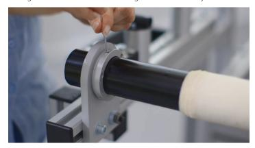
> Tighten the screws of the ratchet wheel with the Allen key and make sure that the backing rail runs smoothly (without play) and doesn't block.
