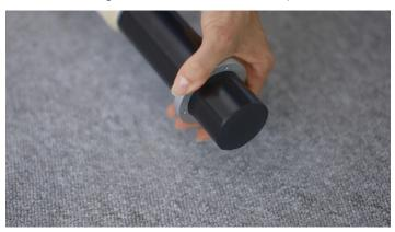
> Pull the ratchet wheel over the right end of the top rail. The cogs of the ratchet wheel point to the back (not to the front) when you stand in front of the Frame! This means that the flange ring with the screws is inwards and not towards the end of the rail.
