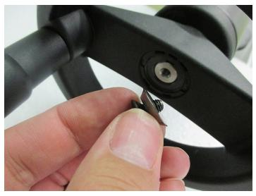
> Cover the screw of the handwheel with the sticker.
