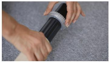
> Position the backing rail centrally into the rail support on each end.
