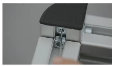
> Place the washer on the screw, insert the screw with the washer from above into the groove of the bar and tighten firmly with the Allen key. The bar and the longitudinal bracing must be at the same height.
