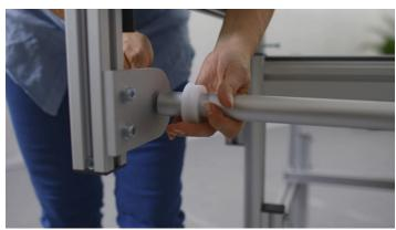
> Pull the ratchet wheel over the right end of the top rail. The cogs of the ratchet wheel point to the front (not to the back) when you stand in front of the Frame! This means that the flange ring with the screws points inwards and not towards the end of the rail.
