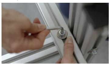
> Place the left edge of the lower bar on the left leg so that the screw hole corresponds with the preassembled slot nut.
