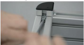
> Insert the spring slot nut from beneath into the groove of the left leg and position it exactly in front of the screw hole.
