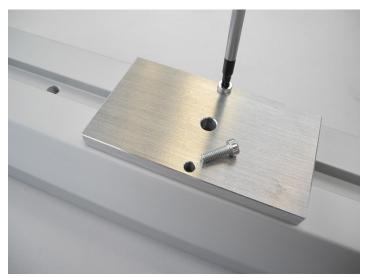
> Attach the rear stand profile on the bottom side of the machine from beneath. For this purpose place the screw P10 and the washer P9 through the hole in the middle of the profile. Tighten the screw placed into the second movable slot nut with the torx screwdriver. This movable slot nut has already been inserted into the groove.
