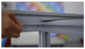
> Place the washer onto the screw, insert the screw with the washer into the left groove of the center leg and tighten firmly with the Allen key.
