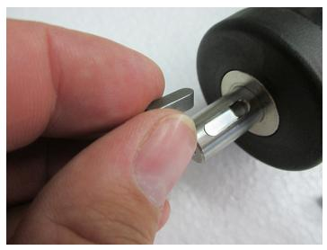
> Position the handwheel exactly on the protruding end.
