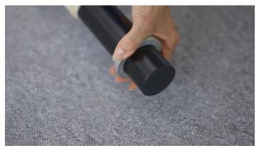
> Pull the ratchet wheel over the right end of the backing rail. The cogs of the ratchet wheel point to the back (not to the front) when you stand in front of the Frame! This means that the flange ring with the screws points inwards and not towards the end of the rail.
