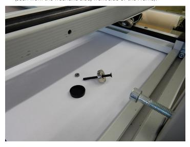
> Push the countersunk head screw through the magnet, insert the screw with the magnet into the hole and tighten the nut.
