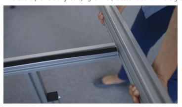
> Put the bar into the groove of the left leg and make sure that the corners of the bar and the longitudinal bracing are flush against each other. This applies to all four corners.
