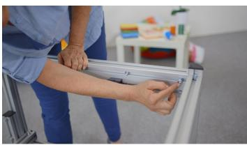
> Position the left rail support from outside in front of the left leg so that the screws can be screwed with the pre-assembled spring slot nuts.
