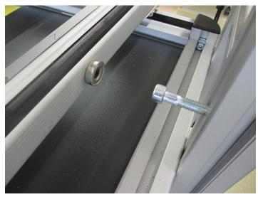
> Make sure that the carriage can be moved easily on the rails and all the wheels are in contact with the tracks. As a check for the best possible contact with the tracks, feel the rollers with four fingers.
