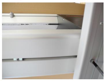
> Now, move the rear stand profile in that direction that the edge of the aluminum plate fits to the position of the arrowhead as shown below.
