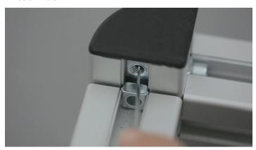
> Put the washer onto the screw, insert the screw from above into the groove of the bar and tighten firmly with the Allen key.
