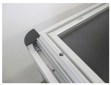
> Align the screw holes of the pre-assembled track, which is in the upper groove of the rear bar, parallel to the screw holes of the track.
