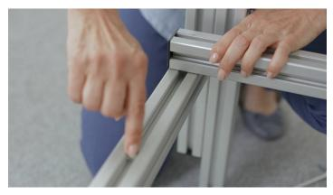
> Tighten the scew and its washer with the Allen key.
