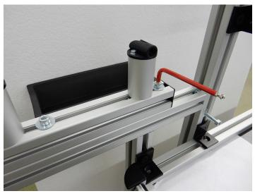
> Push the front part of the movable bracing inwards as far at it will go against the vertical bar.
