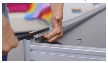
> Tighten the two last screws slightly with the Allen key.
