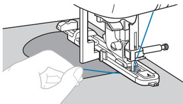
**7 Raise the presser foot lever, remove the fabric, and then cut the threads.**
