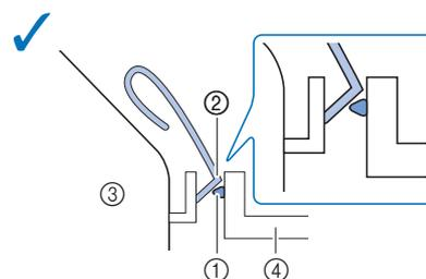
Notch (①) does not fit firmly under the bend in the lever (②).
