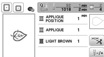
→ The position of the appliqué is sewn, and then the machine stops.
