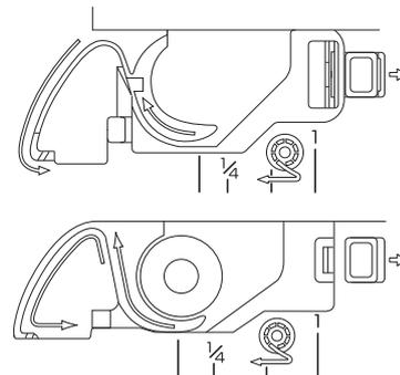
8 While lightly holding down the bobbin with your right hand (①), guide the thread through the slit in the needle plate cover (②) and lightly pull it with your left hand (③).
