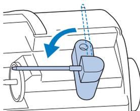
**6 Place the upper thread spool for the needle on the right side onto the spool pin, and then secure it with the spool cap.**
