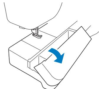
A presser foot accessory tray is stored in the accessory compartment of the flat bed attachment.
