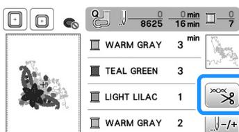
2 Press to turn off the automatic thread cutting function.
