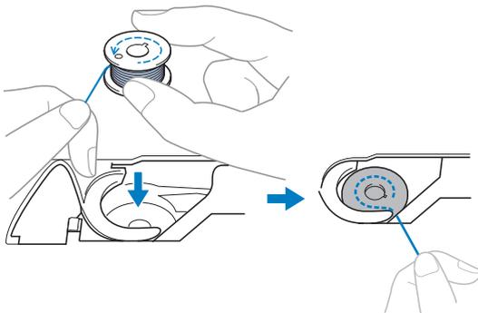
7 Lightly hold down the bobbin with your right hand (①), and then guide the end of the thread around the tab of the needle plate cover with your left hand (②).
