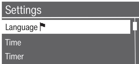
A scroll bar at the right of the display shows that additional options or text are available. Use the arrow keys  $\wedge$   $\vee$  to display them.
