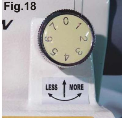
In Fig.18 at left you can see that the arrow at bottom points to the depth setting. Here you can see it is set at “4”.
