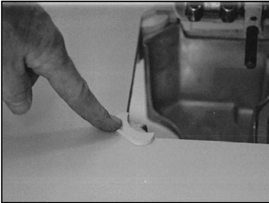
8. Now, turn the table upright. Slide the oil pan rubber corners onto the oil pan and set the pan into the table.
