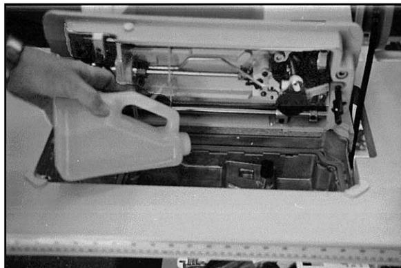
11. Install the machine rest into the pre-drilled hole.
