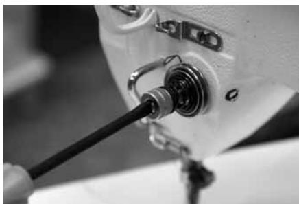
Figure 3-110 For fine adjustment of check spring insert screwdriver turn clockwise for more tension
