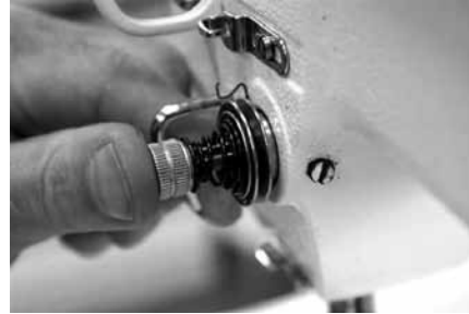
Figure 3-107 Release and the disk will close; this is the proper place for your tension assembly
