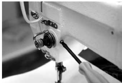
Figure 3-86 Screw on inside of machine LOOSEN ONLY. DO NOT REMOVE
