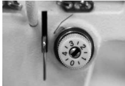
Figure 3-85 Tension assembly with good spring (new tension knob)
