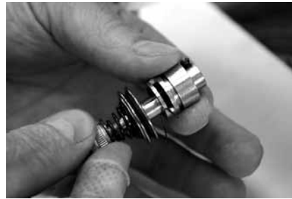
Figure 3-91 Remove tension assembly from barrel
