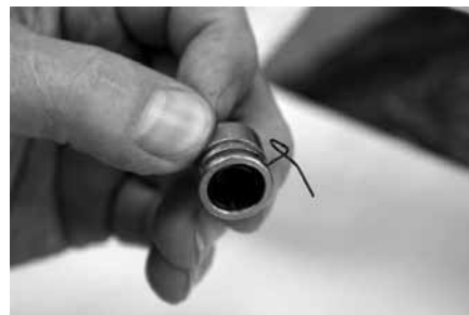
Figure 3-99 New spring in place
