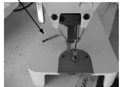
Oil Reservoir with dip stick removed
