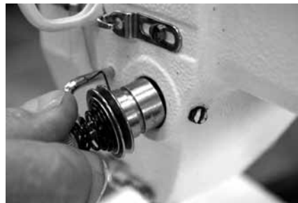
Figure 3-87 Remove assembly from machine. Be careful with release pin
