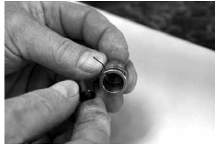
Figure 3-97 Insert the new spring
