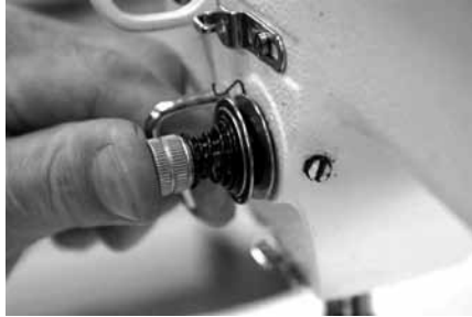
Figure 3-106 Press in and notice the tension disk opens
