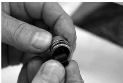
Figure 3-98 Twist while inserting the new spring
