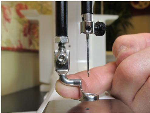
3. Ensure the foot is centered with the needle when the foot is fully tightened with the 2.5mm hex wrench. If it isn't properly centered, loosen the lock nut; center the foot with the needle; hold the foot in position; and firmly tighten the lock nut.
