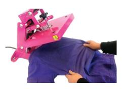
Once the Craft Press has reached the designated temperature, position the garment on the lower platen.
