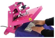
Align the transfer material on the garment to be printed.
