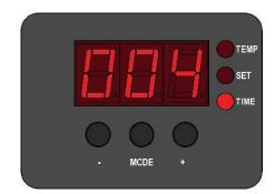
The timer will count down and audibly signal you to lift the heat platen into the UP position when the press cycle is complete. The time will automatically re-set and you are ready to continue with the next application.
