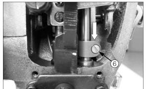
► Manually turn the pulley to locate the needle bar at the lowest point. Loosen the screw® of the needle bar.
