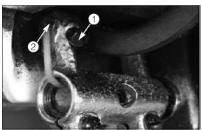
► When the feed dog is at the highest position, turn the feed dog turning shaft② to make the upside face of the feed dog horizontal with the needle plate.
