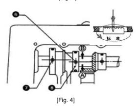
When the feeding distance dial is set at the maximum position, when the feeding tooth drops from the highest position, the center of the machine pinhole should be at the same level as the front 1-2 teeth of the feeding tooth on the surface of the needle plate
