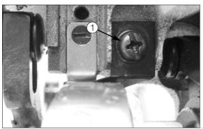
► Loosen the fixing screw① for the thread retainer.
