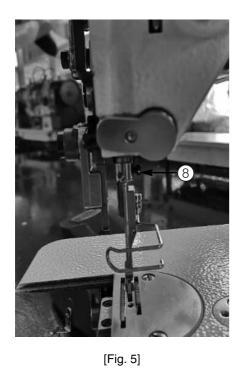
► Turn the pulley to set the needle bar® at the highest point.
