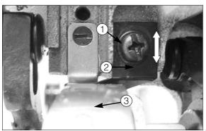
► Move the thread retainer② up and down to make sure that the moving mes④ and the hook ③ don't interfere with each other and then tightly tighten the fixing screw①.
