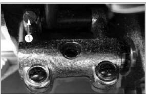
$\blacktriangleright$  Loosen the fixing screw 1 for the feed dog support shaft.
