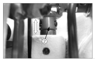
► Slightly move the upright shaft upper gear② up and down, and check the clearance of the upright shaft.
