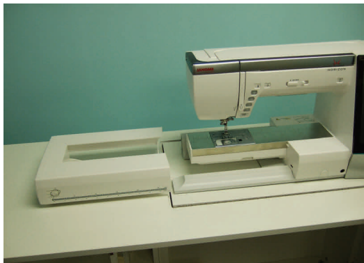
Janome 15,000 in freearm position, top of cabinet showing how to remove the accessory kit for best fit on platform. Custom made, machine specific acrylic insert is available as optional accessory.
