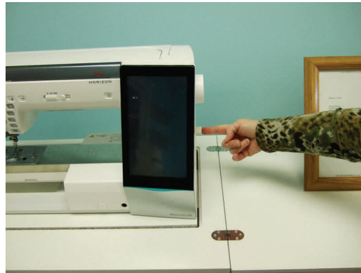
Note that when the right side of the sewing machine base is at the right edge of platform, the differential control knob and hand wheel extend further to the right than opening allows. Cords not plugged in. Push down on machine and platform to lower unit slowly. When you hear a click and stop in flatbed to reposition the machine to the left as shown next.
