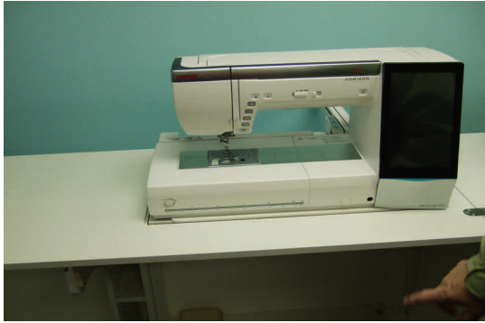
Janome 15,000 on Aussie Cabinet platform. Knee lifter lever cannot be used. Lift supports the weight of machine.
