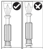
Screw cam bolts flush as illustrated.
