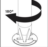
Press cam Into hole until flush with Insert bolt through pre-drilled Turn clockwise to lock cam with bolt.
