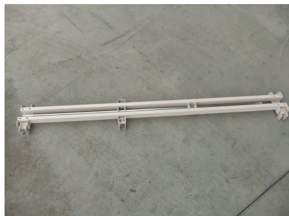
2. Support Frame — sub assembly
