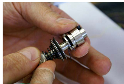
Figure 3-91 Remove tension assembly from barrel
