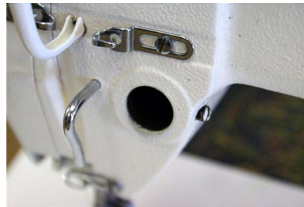
Figure 3-88 Machine with tension assembly re- moved
