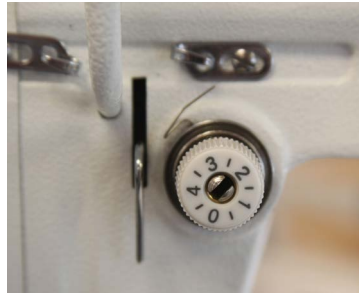
Figure 3-85 Tension Assembly with good spring (new Tension knob)
