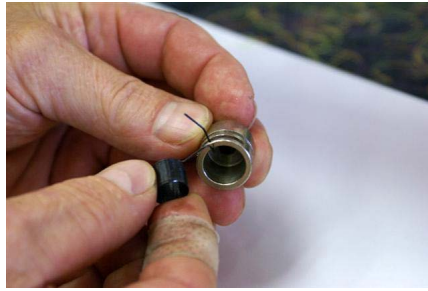
Figure 3-97 Insert the new spring
