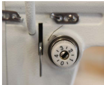
Figure 3-109 Tension assembly back in place with new check spring at 11:00
