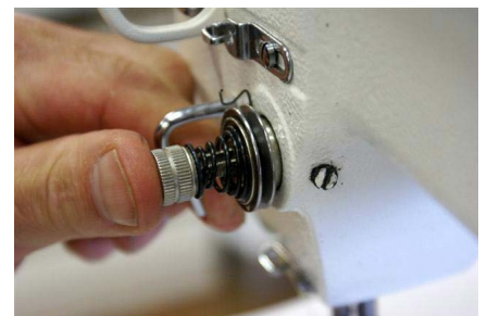
Figure 3-107 Release and the disk will close; this is the proper place for your tension assembly
