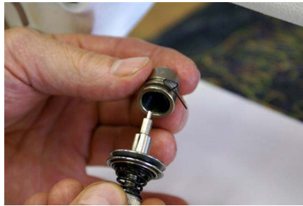
Figure 3-100 Insert the tension assembly back into the barrel. REMEMBER DO NOT LOOSE THE PIN
