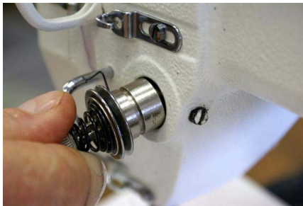
Figure 3-87 Remove assembly from machine Be careful of release pin
