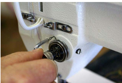
Figure 3-105 Once in ensure that your check spring is at 11:00
