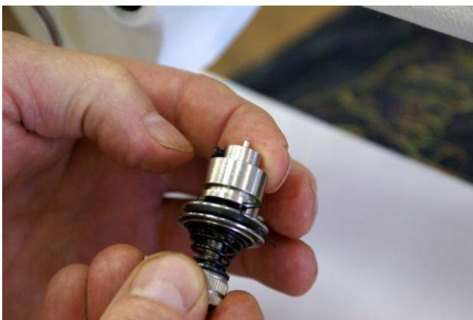
Figure 3-102 Give the tension assembly a twist until you feel resistance on the check spring
