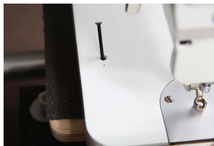
Figure 3-3 Oil dip stick lifted
