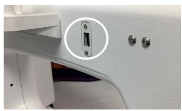
Machine large USB connection for front handlebar large connector
