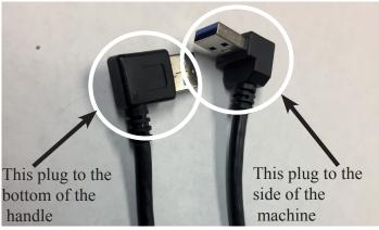
QM23011 Handlebar to machine large USB cable
