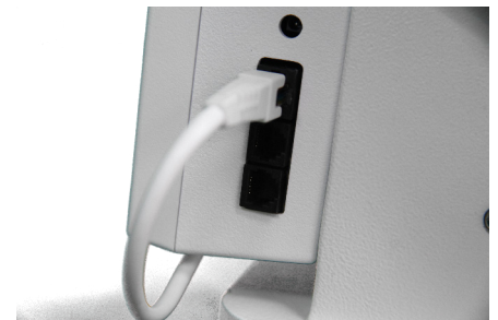
Backside of main power supply where the encoders and handlebars connect
