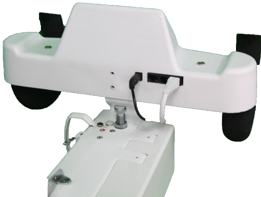
Backside of handlebars showing where to connect cables
