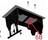
6B - Once table is assembled, hold center support(s) under table top with drill holes aligned and drill downward from table top into center support(s)
