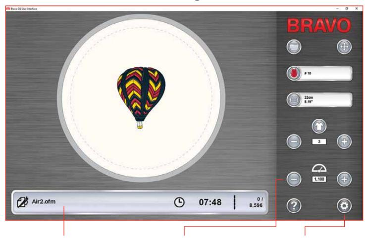
Colorized machine status indicator (ready, running, stopped) for easy monitoring. Remaining sew time and stitch count are clearly displayed.
