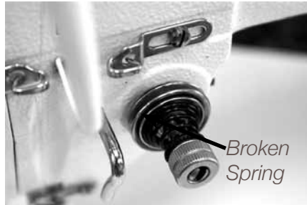
Figure 3-84 Tension assembly with broken spring. (old tension knob)
