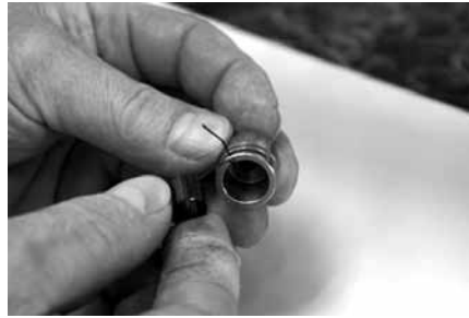
Figure 3-97 Insert the new spring
