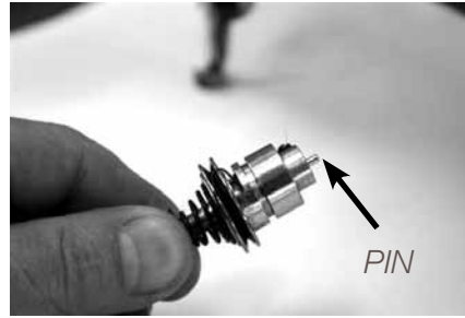
Figure 3-89 Tension assembly out of machine DO NOT LOSE PIN
