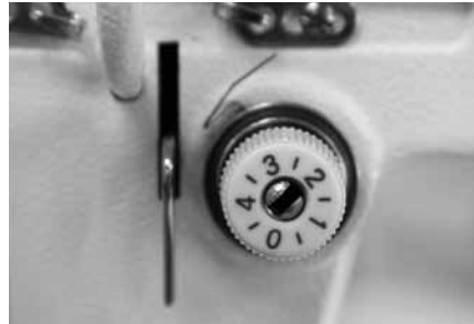
Figure 3-85 Tension assembly with good spring (new tension knob)
