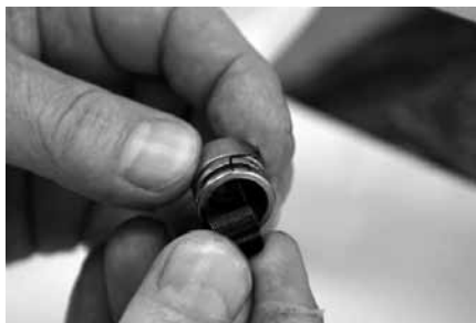
Figure 3-98 Twist while inserting the new spring
