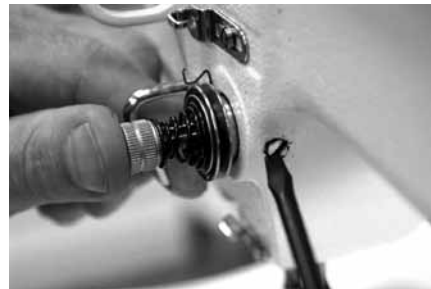
Figure 3-108 Tighten screw on your machine
