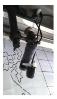
The cable can go over the top of the lower arm secured by a clip or if your machine allows under the lower arm. Face the clip with the opening towards the back of your machine to secure the wire. Attach camera to the cable.
