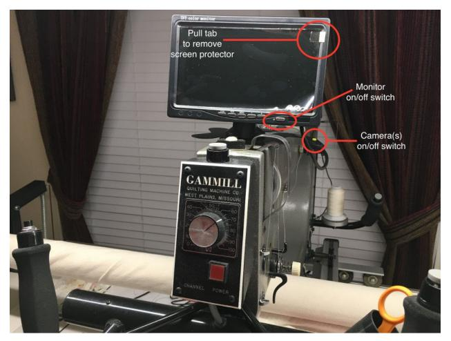
Once the monitor is mounted, we're going to start feeding the cables through the provided clips starting at the top by anchoring the cable a few inches past the camera on/off switch (yellow button).
