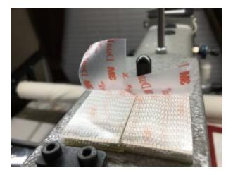
Press 2 more strips of the dual lock to those you have already applied, peel away the backing and firmly press the monitor in place onto the dual lock strips.
