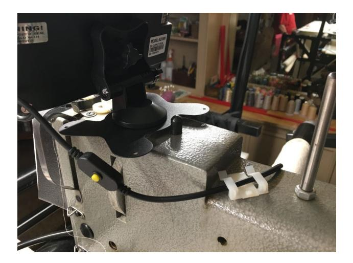
The two camera cables have been tied together. Remove the tie and take the cluster of cables tied with the black tie and untwist.
