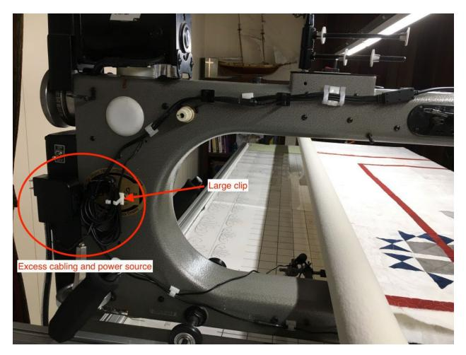
Find the power source in the box. Locate where you would like to place it on your longarm (on the back side, towards the back, etc.). Place one strip of dual lock vertically onto the power source. Then place a second strip of dual lock onto the strip you've already placed, locking it in. Peel the backing and press the power source firmly onto the longarm. \*\*You will need to provide your own extension cord with a length long enough to accommodate the movement of your machine.
