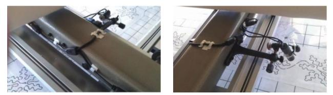
Push the V2 button on the monitor screen and adjust the angle and position of the camera so that your view is following the laser light.
