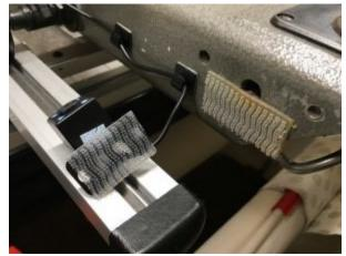
Connect the yellow end of the cable to the yellow end of the stitch camera.
