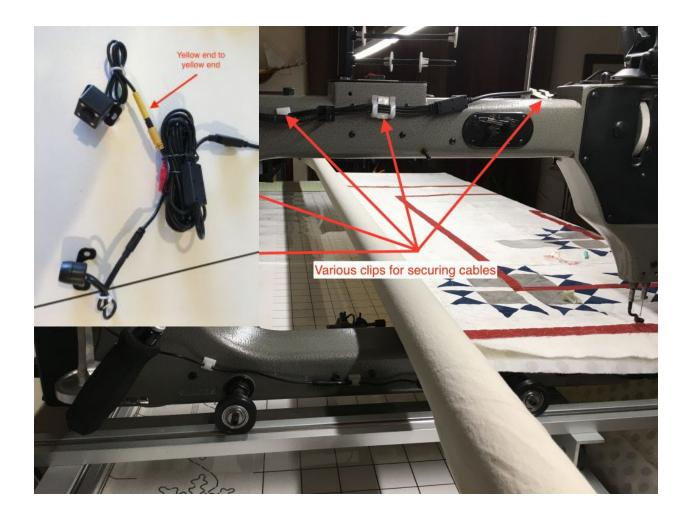
Take a piece of dual lock and attach it to the bracket of the stitch camera (camera with four small LED lights).
