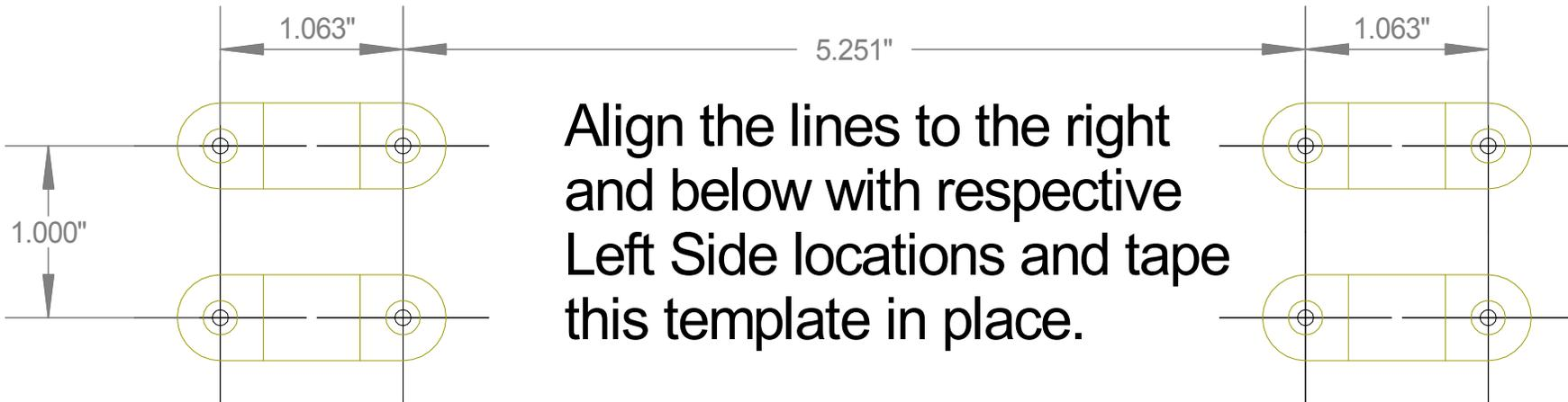
Align the lines to the right and below with respective Left Side locations and tape this template in place.
