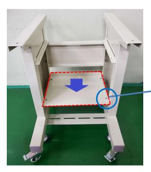
① Place the bottom shelf at the low position as shown in the picture. (Note: the bottom shelf has 4 mounting holes)
