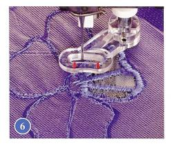
When using the free-motion quilting foot, let the marks on the front ring guide you when sewing. The maximum left/right needle swing is between the marks. Center the design lines between the marks keeping the design straight or parallel to the front of the machine.
