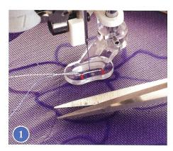
2. Select the straight stitch, center needle position, and outline stitch following all the design lines. Stitch around each section a second time. (#2)
