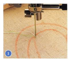
Lower the feed dogs and bring the bobbin thread to the top and lockstitch the threads. Trim the thread tails before stitching. (#1)
