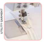
An invisible zipper is always inserted before stitching the garment seam. The Invisible Zipper Foot has two grooves underneath the foot to accommodate the zipper coils and hold them in place as you stitch.
