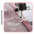
Insert package piping into seams and edges for a tailored finish. Cover cord with fabric for specialty piping. The clear view allows you to see the piping placement and see exactly where you are stitching and enables you to see the first row of stitching and adjust your needle position to
