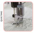
The Open Toe Free Motion Spring Foot gives clear visibility when doing free motion quilting or embroidery. Because of the open front, you can easily do stippling or follow a design in the fabric. The spring action keeps the fabric from lifting with the needle as the stitch is being formed
