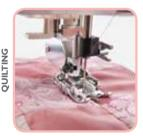
Use the Changeable Quilter's Guide Foot when stitching in the ditch along a seam line. The foot has guidelines to make it easy to accurately turn corners for 1/4 (6mm) or 1/8 (3mm) seams.
