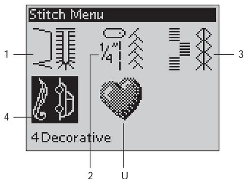
The name and number of the selected menu is shown at the bottom of the display. The stitches are pictured inside the lid of your machine with the menu numbers on the left and the stitch numbers within the menus across the center.
