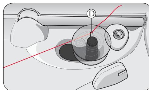
*Note: When using earlier version of HUSQVARNA VIKING® bobbins that do not have a hole, wind several turns of thread on the bobbin to get started.*
