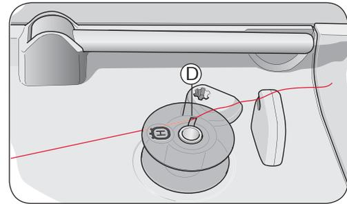
*Note: When using earlier version of HUSQVARNA VIKING® bobbins that do not have a hole, wind several turns of thread on the bobbin to get started.*
