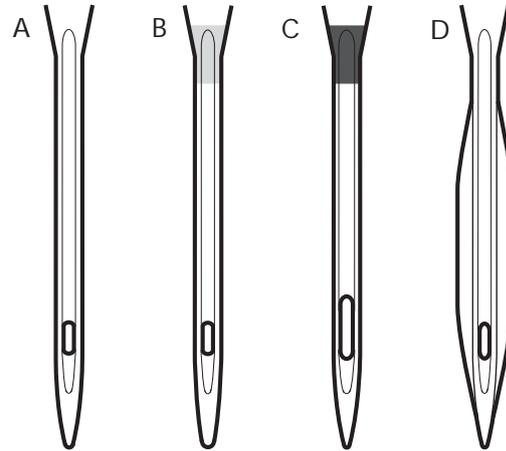
*Note: Change the needle often. Always use a straight needle with a sharp point (1). A damaged needle (2) can cause skipped stitches, breakage of needles or snapping of thread. A damaged needle can also damage the stitch plate.*
