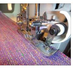
seaming, trimming, and overcastting with one pass under the needle(s)
